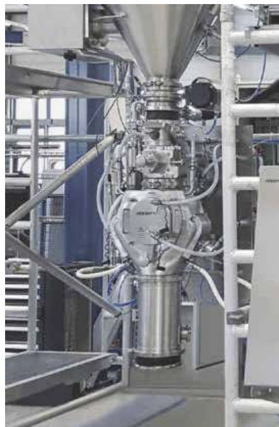
Hammerwitt-6 hammer mill with dosing unit
