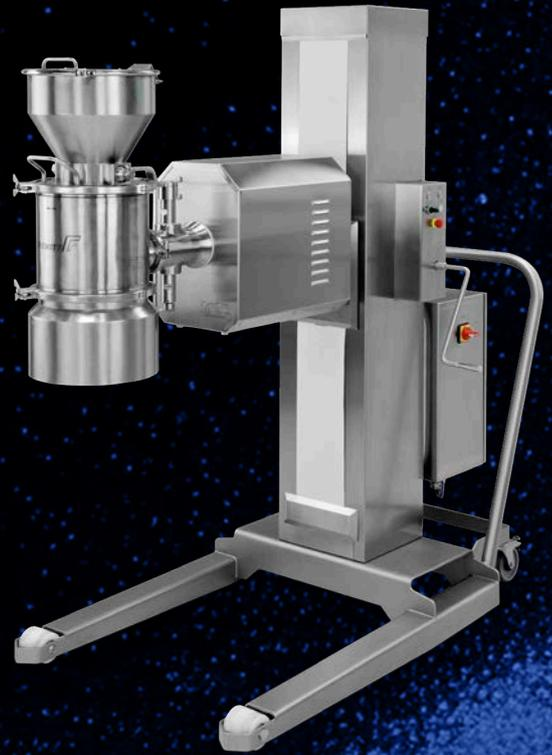
The EasyMill RS-200 is a rotary cylindrical sifter, designed for the de-agglomeration and homogenization of any type of powder, dry or wet.
